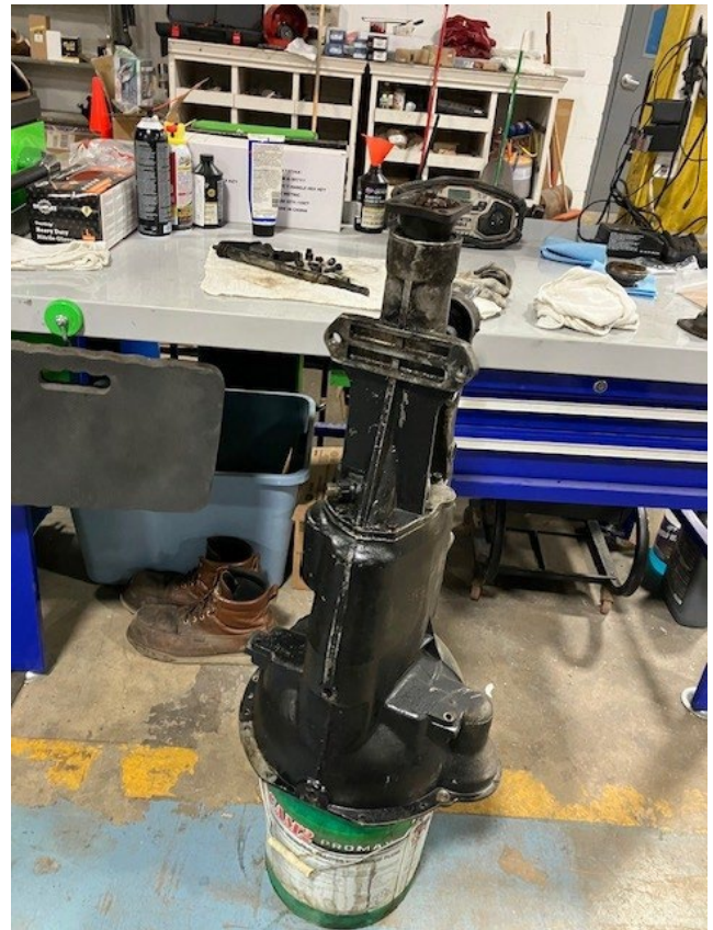
Success – tranny is out, front seal is out, and remaining oil is draining into a bucket!
