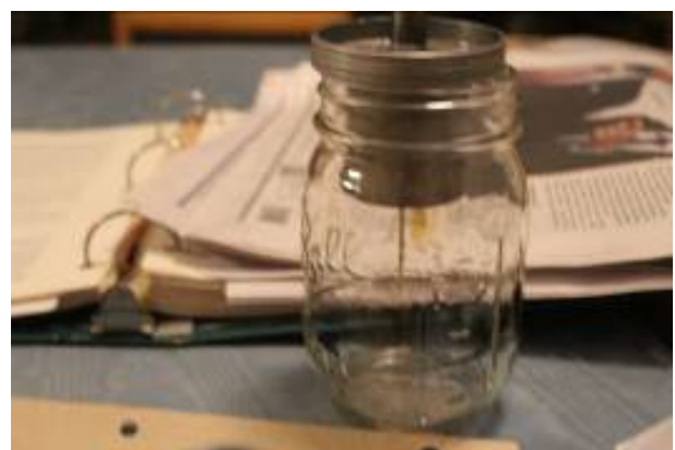
Figure 2: Piston and fuel needle in a Ball Mason jar, which keeps the needle safe from bending.
