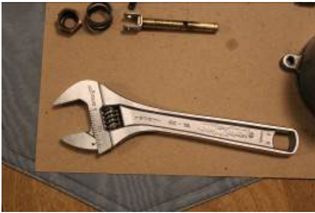
Figure 3: New wrench (Channel Lock, 6", with graduations to set the Jaw gap, full open is 0.94in.. Cost was $17 at Menard's. Needed tapered jaw width to fit Jet locking Nut...
