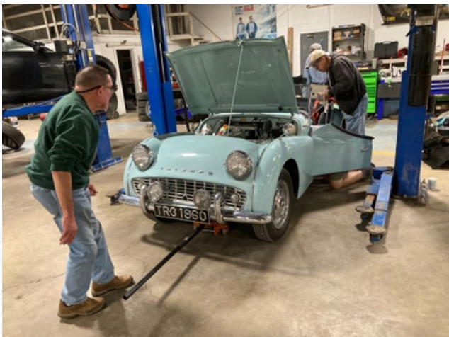
Stan jacking up the engine to free the tranny.
