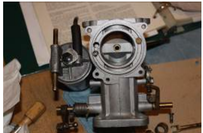
Figure 1: Top of carb. Looking across the air passage at the fuel bridge. Fuel float bowl is to the left.
