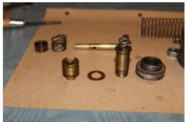
Figure 7: Foreground, Top half jet bearing, copper washer, bottom half jet bearing with spring inserted, Jet locking nut with cork seal on top of a copper washer (dark line under cork).
