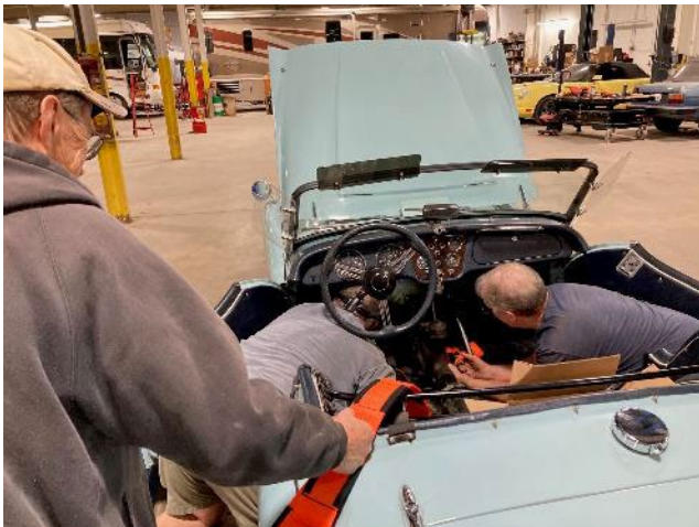
Bruce and Harry removing the bolts connecting the engine and tranny while chuck readies the lifting strap.
