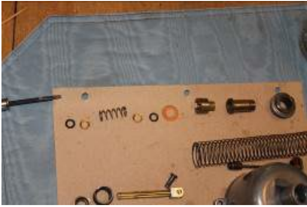
Figure 8: O-ring seal (probably Nitrile material) which now replaces the original cork seal, copper washer for between seal and spring, spring, copper washer for end of spring, O-ring seal. Hard to see, but copper washers have beveled surface on seal side, these 5 parts fit into the bottom half jet bearing which is third piece after second O-ring.
