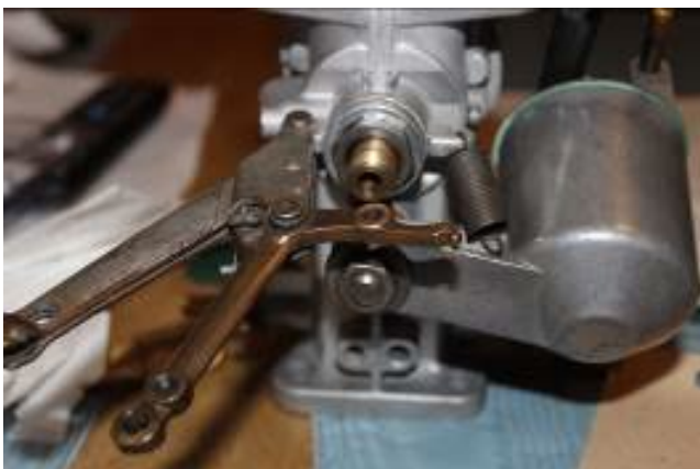
Figure 5: Looking up Jet fuel passage. Jet Adjusting Nut and Spring removed. Bottom Half Jet Bearing and Jet Locking nut are visible. Fuel float bowl is on right.
