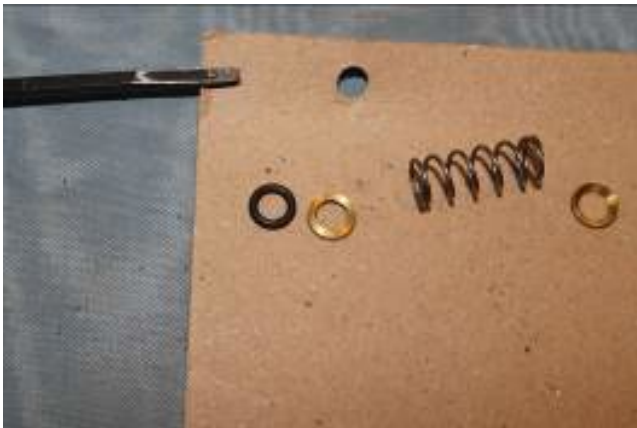
Figure 9: copper washer turned over to show flat side that fits up against the spring when correctly assembled.
