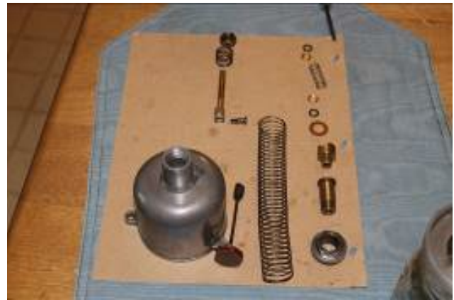
Figure 6: Jet Fuel Passage parts layout. Foreground – Vacuum dome, Damper assembly and spring which loads piston and fuel needle (in Mason jar). Background left, clevis pin, Jet head, short spring and Jet adjusting nut. On the right, near to far: Jet locking nut, Bottom half Jet bearing, top half Jet bearing, copper washer, O-ring, copper washer, spring, copper washer and O-ring.
