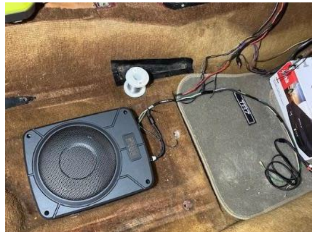
Passenger side subwoofer in the midst of being wired-up.
