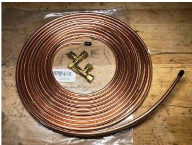
Copper-clad steel fuel (they also list it as brake) line and a couple of true compression "T"s
