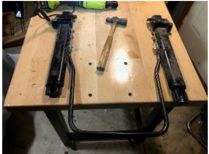
Driver's side seat rail - hammer was needed to take out a dent in the rail that was hampering operation.
