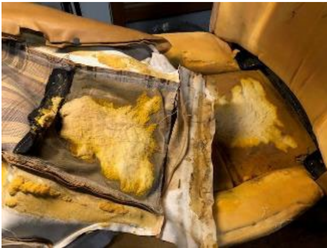
Seat bottom with ripped-up padding glued to it on the left, hole in the padding to the right. Nasty.
