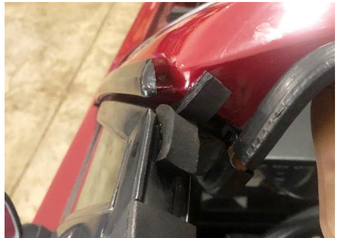
Door closed - good contact with the seals
