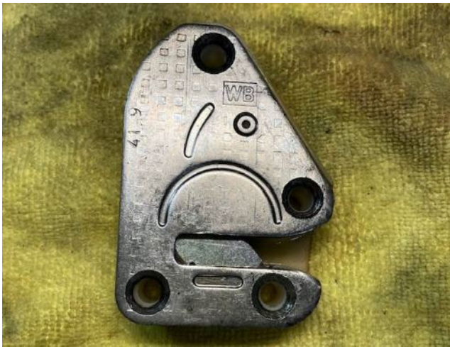
Latch outside – not much wear, or even scuffing, seen
