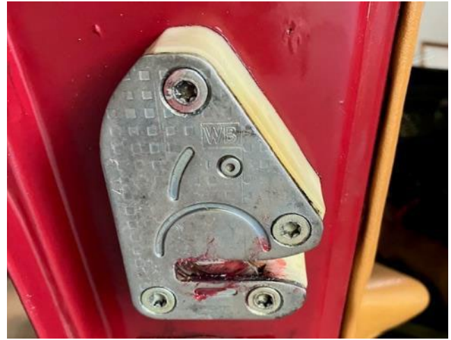
Latch installed and aligned to the existing witness marks
