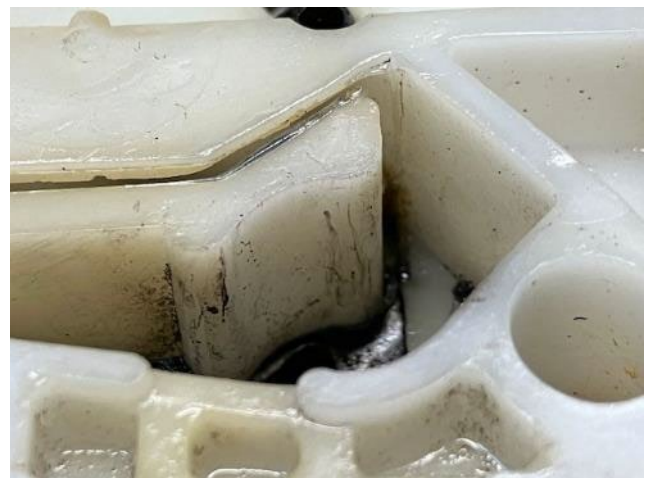
Close-up of the plastic appendage where it normally breaks, between the lobes
