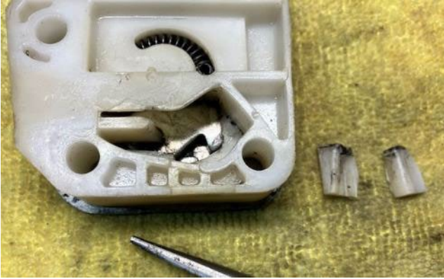
Success – appendage broken off
