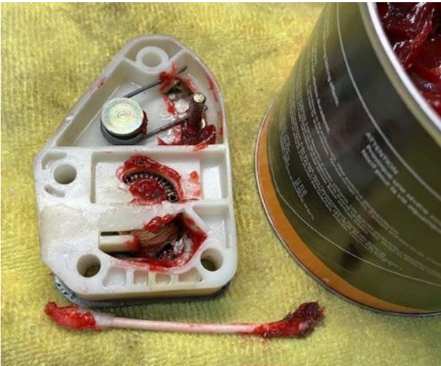
Greased up latch and ready to go back on the car.
