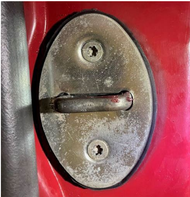
Final location of bottom catch
